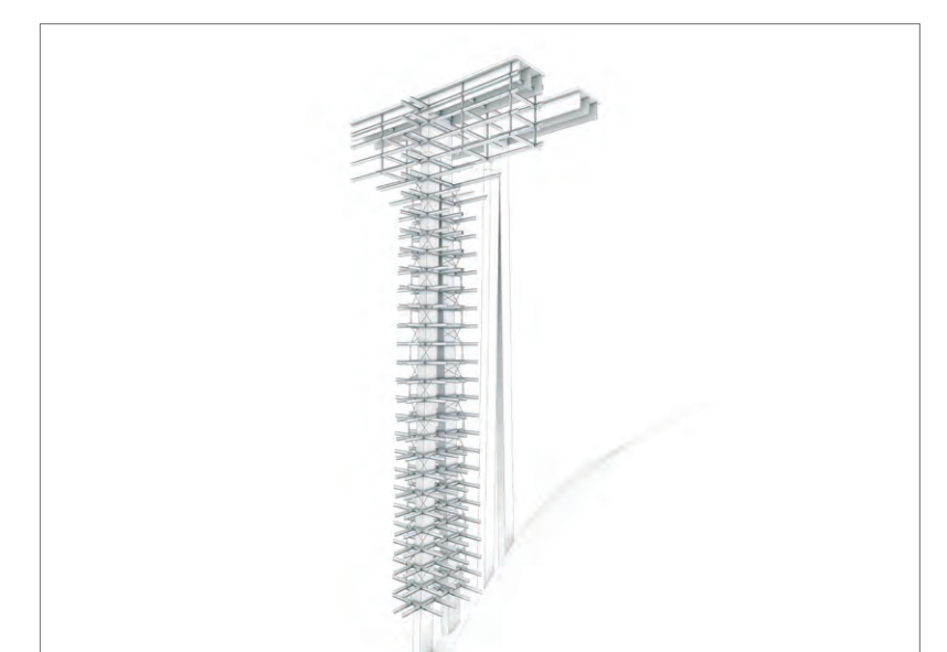
Reinforcement of the structure.
