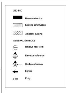
Do not scale this drawing. Figured dimensions only are to be used in preference to small scale drawings. All dimensions are to be checked on site before any work proceeds. Any errors or omissions are to be reported to the designer. If in doubt ask.
